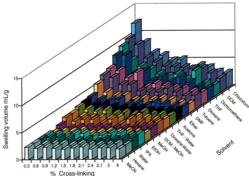
**Figure 3.** Swelling of 0.3–6.0% DVB cross-linked PS resins in a number of different solvents.
