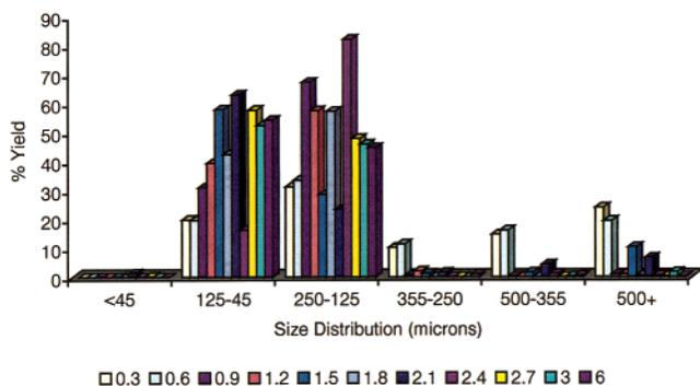
**Figure 2.** Size distribution of the 0.3–6.0% cross-linked beads following suspension polymerization.
