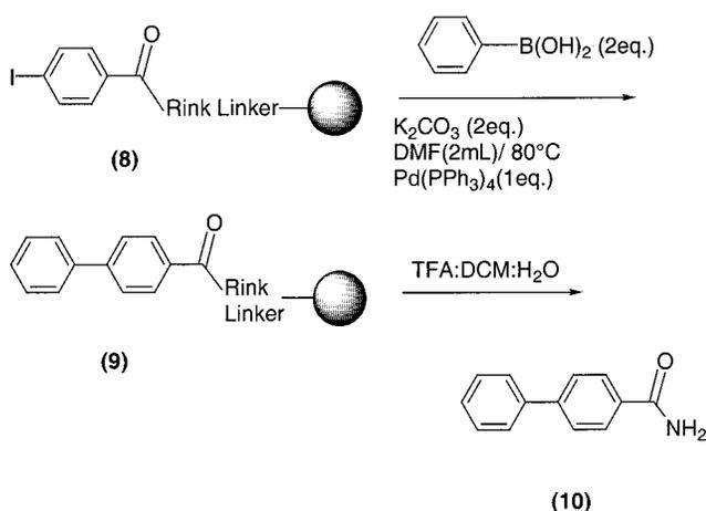
resin cross-linking. The initial rate of biaryl coupling with the 0.3% cross-linked resin was 47 times that of the 6.0% cross-linked resin, representing the accessibility of reactants to the polymeric matrix in a manner that parallels the Methyl Red cleavage.
