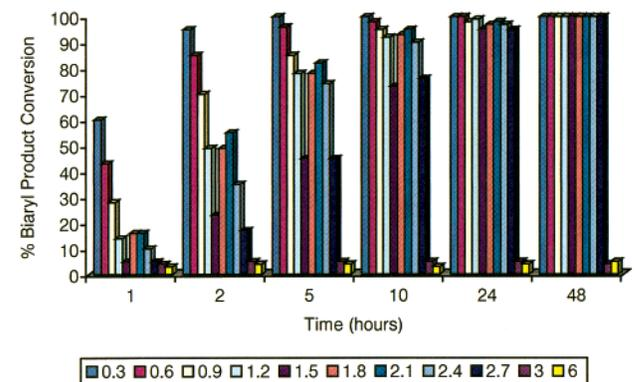
**Figure 7.** Suzuki reaction between phenyl boronic acid and the resin loaded 4-iodobenzoic acid.
