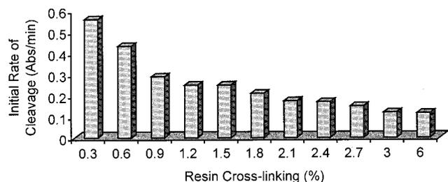
**Figure 5.** Initial rate of Methyl Red carboxamide cleavage reaction vs resin cross-linking.
