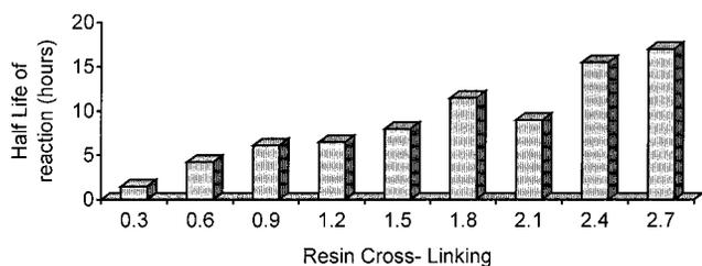
**Figure 8.** Half-life of Suzuki reaction of phenyl boronic acid and Rink loaded 4-iodobenzoic acid on the nine cross-linked resins.
