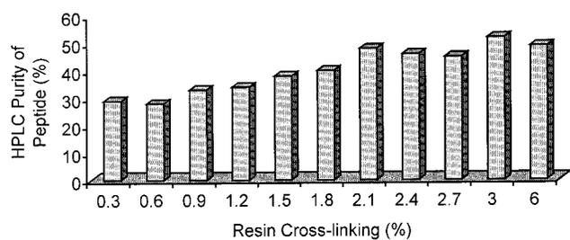
**Figure 6.** Purity of Kawaguchipectin B synthesized on various cross-linked resins (HPLC analysis).
